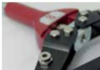
Nose pieces for changing inserted in the tool.
